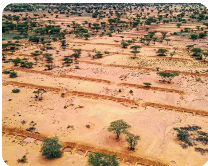
Soil and water conservation through construction of soil bunds in Duruqsi and Mureec villages.
