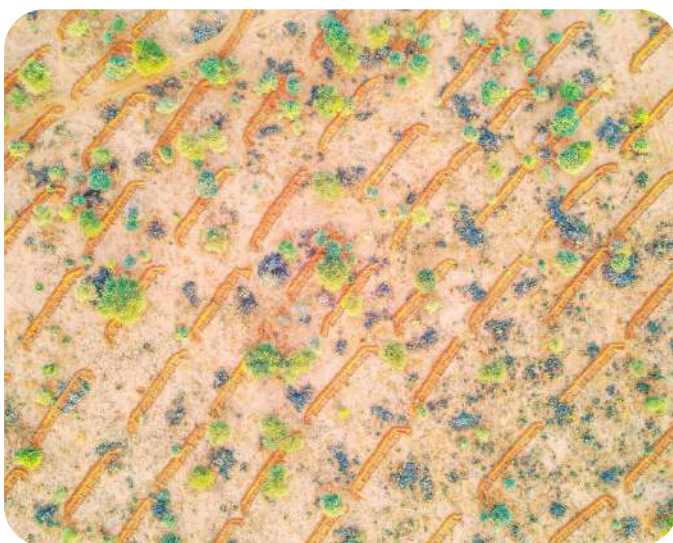
Soil and water conservation through construction of soil bunds in Duruqsi and Mureec villages.
